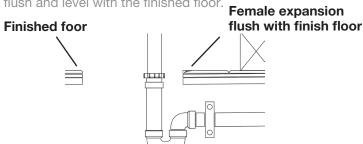
Once in place and flush with the finished floor – secure the female expansion joint and P-trap to a floor joist with a steel-strap to hold it in place.
